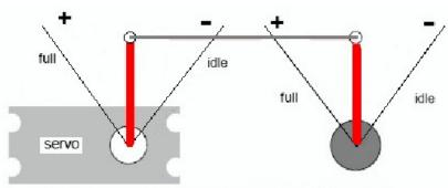
Set-up at half throttle, servo arm same length as carb arm High and Low ATV/End-Points should be as close as possible to the same number
